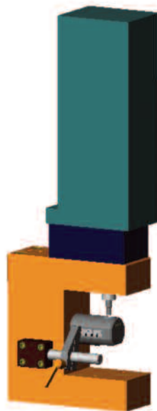
141-RLA-50 Pneumatic single-action unit Throat depth range A = 50 mm Cylinder force 80 kN with air supply pressure of 8 bar
