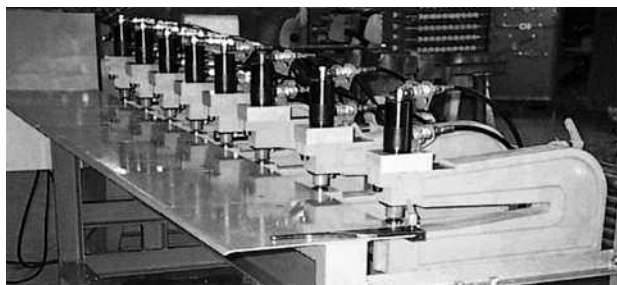
Hydraulic short-stroke cylinder to operate punching units as series punch installation.
