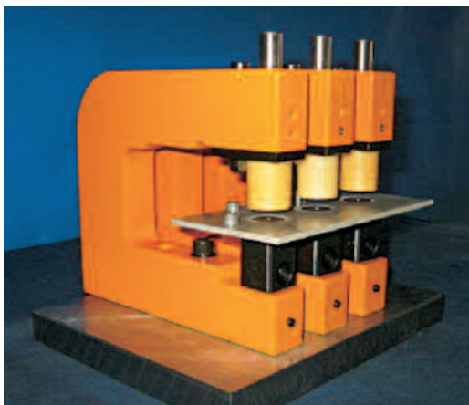
Punching units positioned with a template
