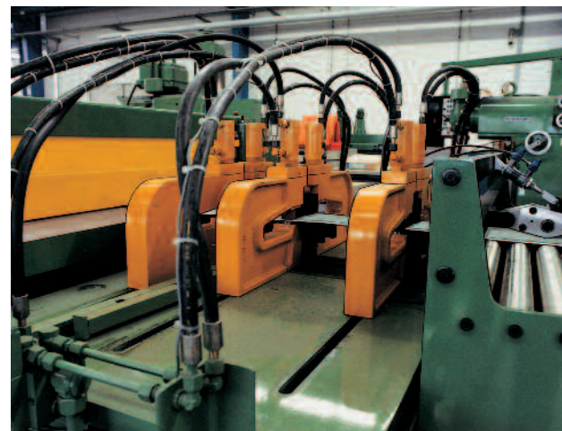
Hydraulic double-action punching units mounted on movable elements for punching steel from coil strips in different widths.
