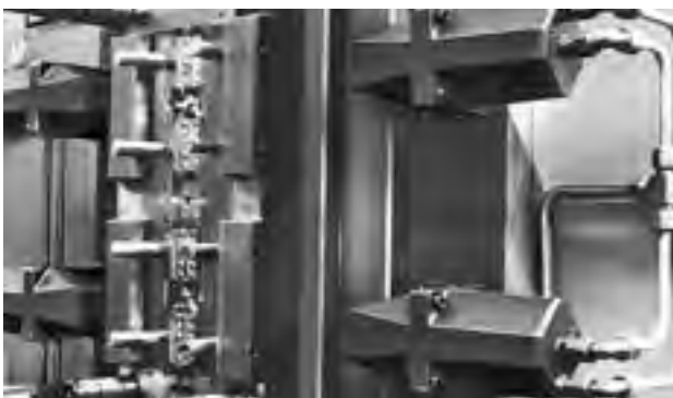
Hydraulic retraction clamp, double action (catalogue page 24.5) for clamping a mould tool to an injection mould machine.
