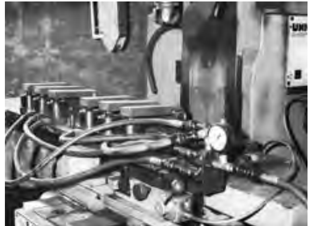
Hydraulic hollow piston cylinder, single action (see catalogue pages 23.13 and 23.14) as a clamping device on a milling machine.
