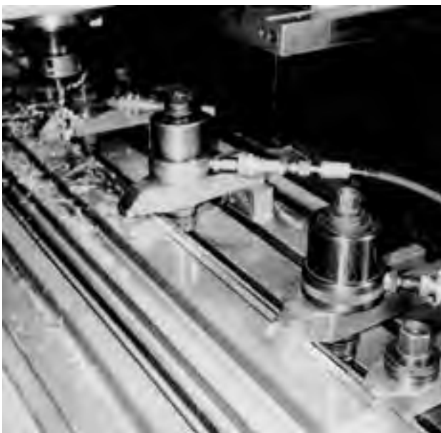
Hydraulic hollow piston cylinder, single action (see catalogue pages 23.13 and 23.14) for clamping on a drilling jig.
