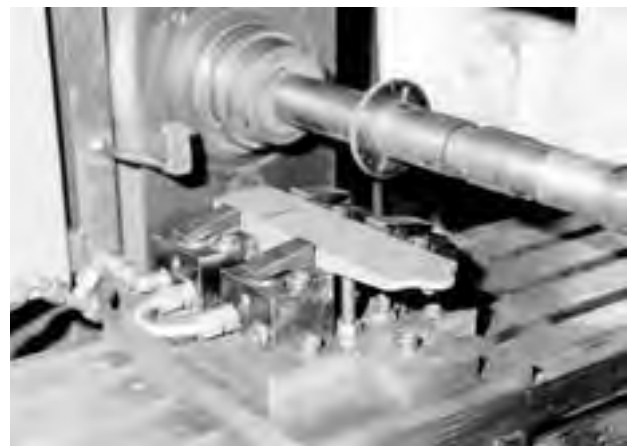
Hydraulic Edge clamp, single action (page 24.7 to 24.8) for clamping on a milling machine.
