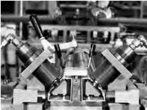
Hydraulic screw-in cylinder, double action (see catalogue pages 23.1 and 23.2) for clamping profiles fixed on a milling machine.
