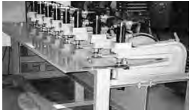
Hydraulic short-stroke cylinders for DE-STA-CO punching units in a series punching fixture
