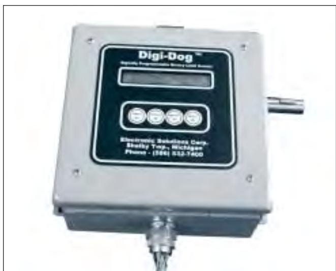
The Digi-Dog is a digitally programmable rotary limit switch based upon resolver technology and EEPROM memory. The Digi-Dog is easily programmed using the operator display. Process times and sequences can be optimized in much less time when compared to other devices. The panel mount allows debugging to occur at a safe distance from the machine. The
