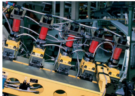
Stamping units placed in line
